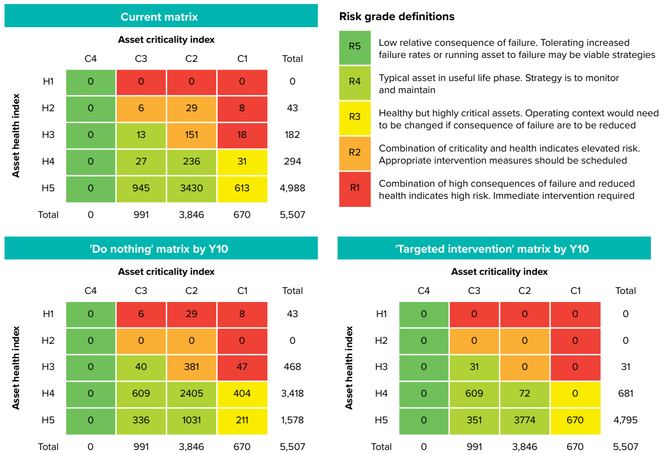
Figure 7.4.7 Subtransmission pole risk matrix
