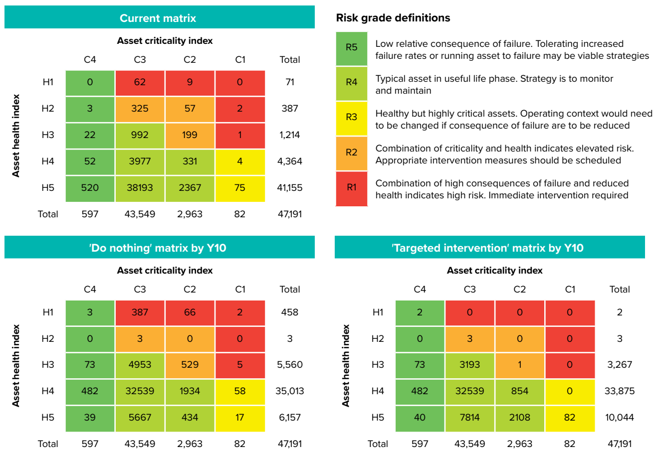
Figure 7.5.6 11kV pole risk matrix
