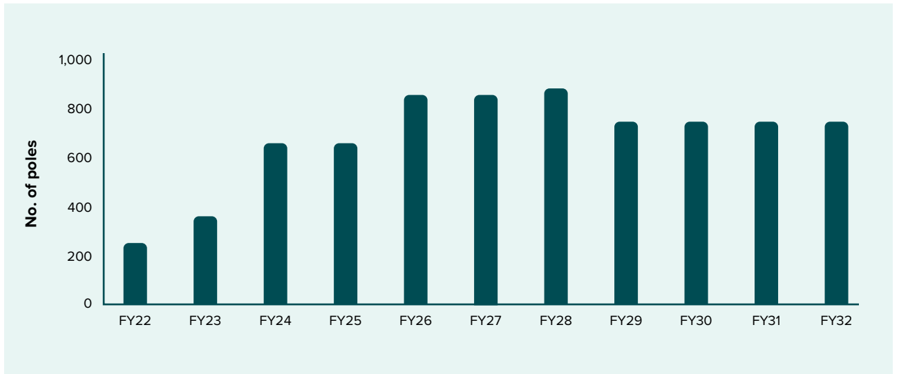
Figure 7.5.8 11kV pole replacement plan
