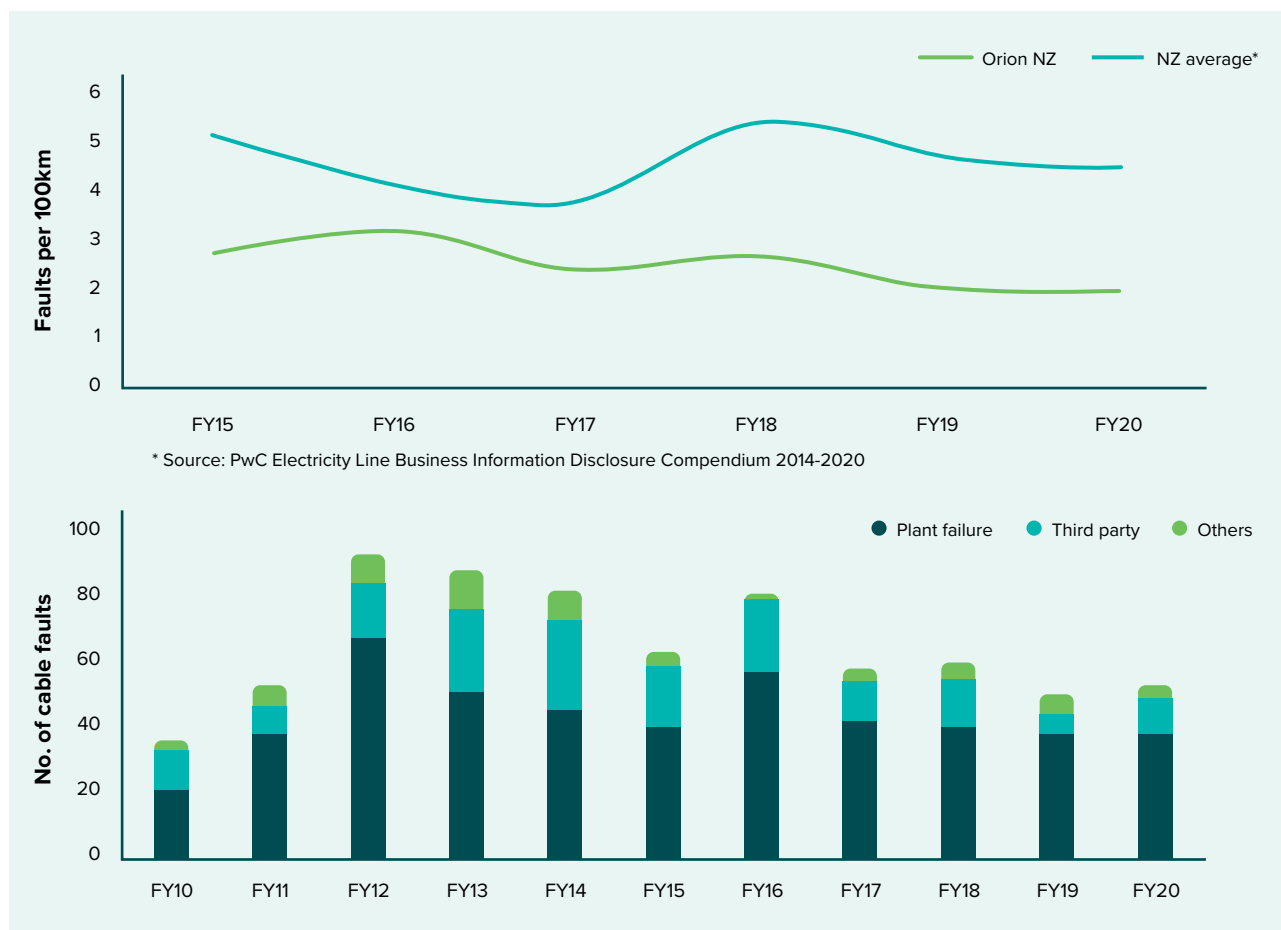
Figure 7.8.2 Number of 11kV underground cable failures and the corresponding SAIDI and SAIFI
