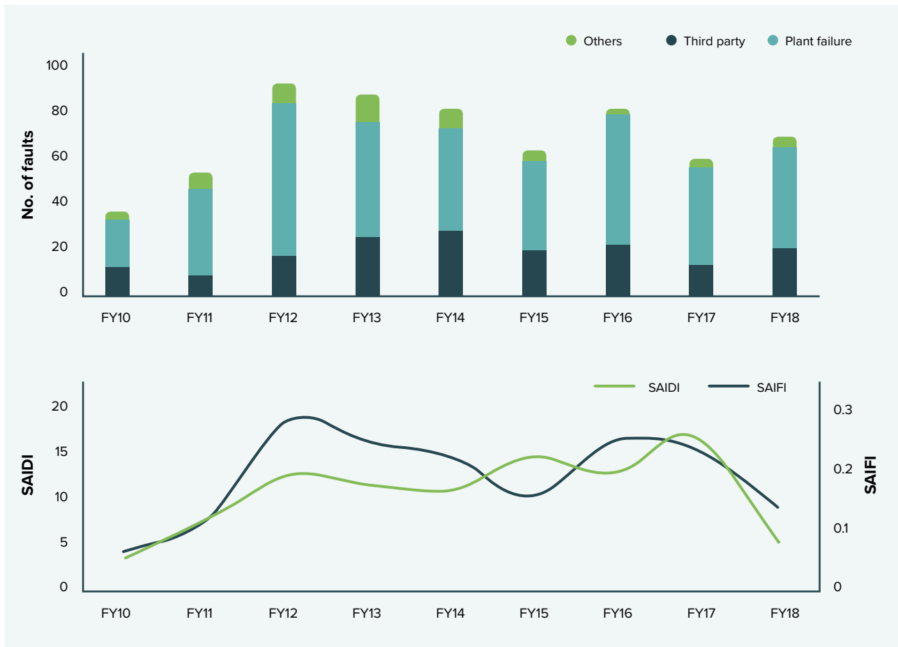
Figure 7.8.2 Number of 11kV underground cable failures and the corresponding SAIDI and SAIFI
