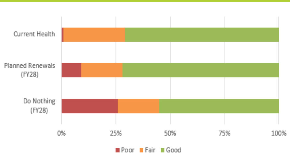
Figure 4-15c Total switchgear 11kV - health index profile
