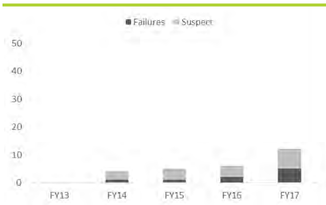
Figure 4-8a - Number of suspect poles and pole failures
