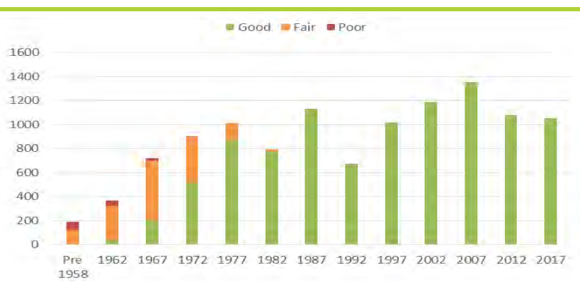
Figure 4-17c Distribution transformers (all) - age/health profile
