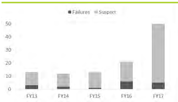
Figure 4-9b - Number of 400V pole failures and suspect poles
