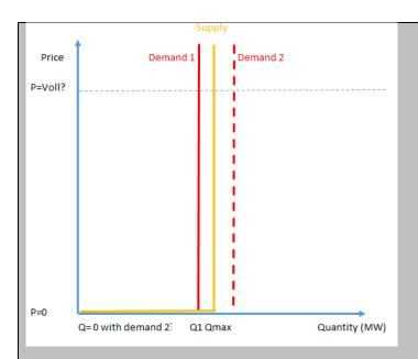
The first thing to note is that there is no supply curve as such. The network has a certain capacity, and in the short term this cannot be changed. Up to this capacity, the SRMC-based price is effectively zero as the available capacity can be 'produced' at zero marginal cost. Once capacity is exceeded it is difficult to say what an appropriate SRMC of supply is, but VoLL would seem the best candidate.<sup>17</sup>
