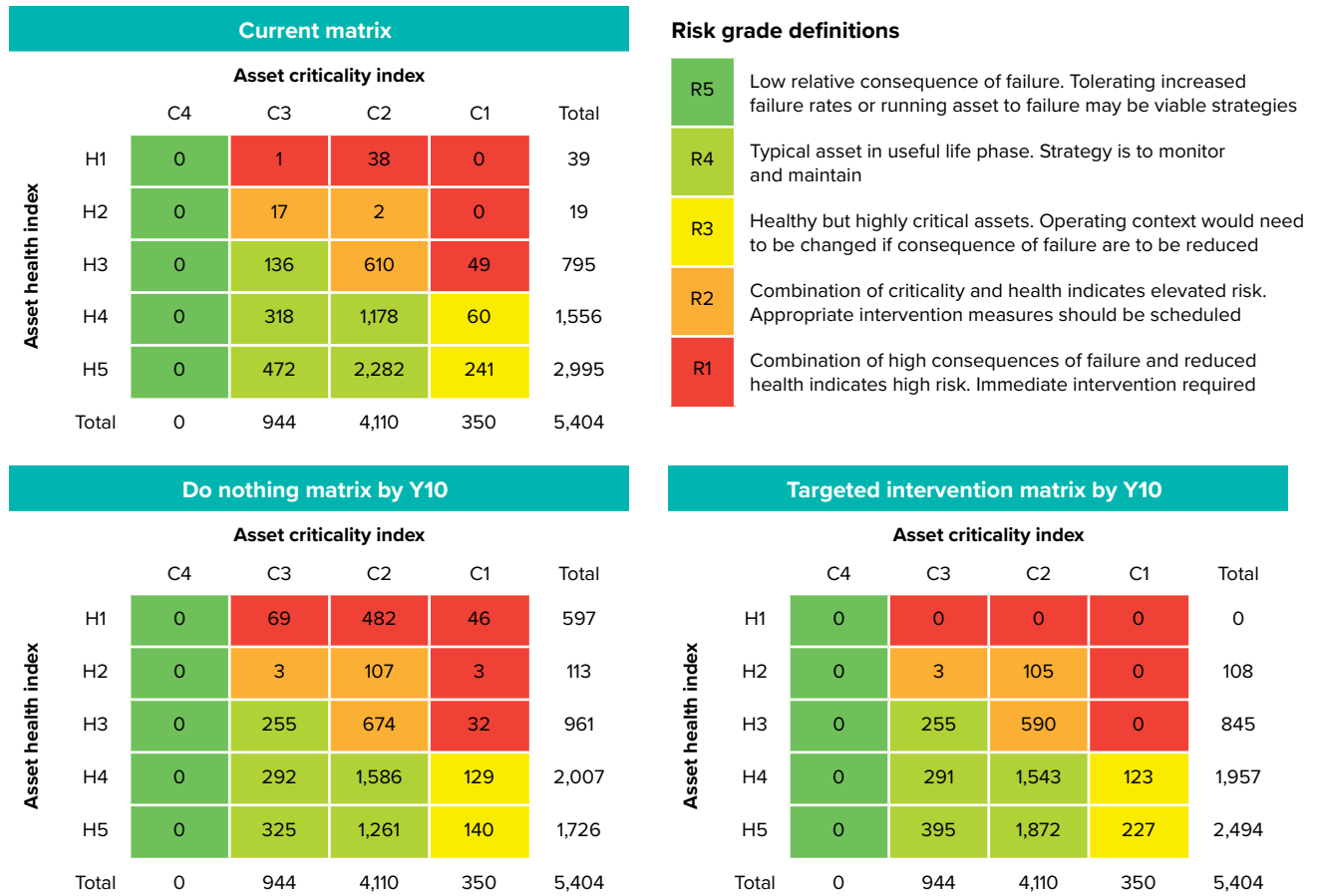
Figure 6.4.7 Subtransmission pole risk matrix
