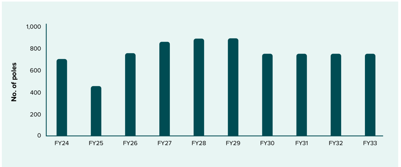
Figure 6.5.8 11kV pole replacement plan
